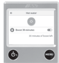
Fig 6. Set up hot water production
