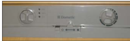
Energy selector switch
